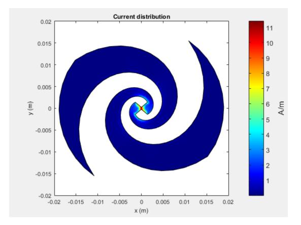
The patch also shows the current distribution of the classic  $\lambda/2$  open-open resistor. The two ends of the patch represent an open circuit since the current is at a minimum.
