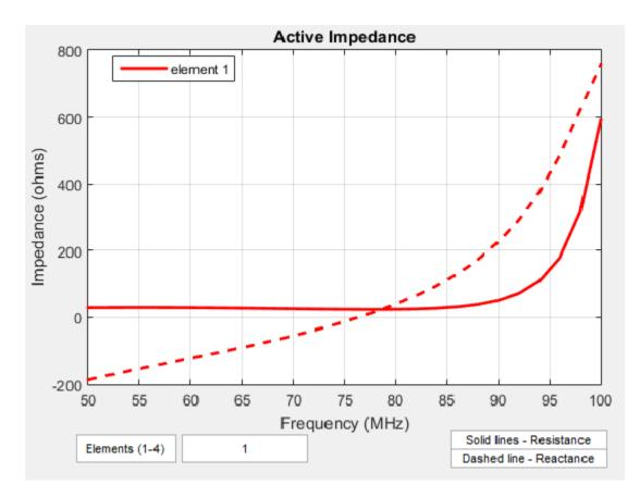
The active impedance of an array depends on:
