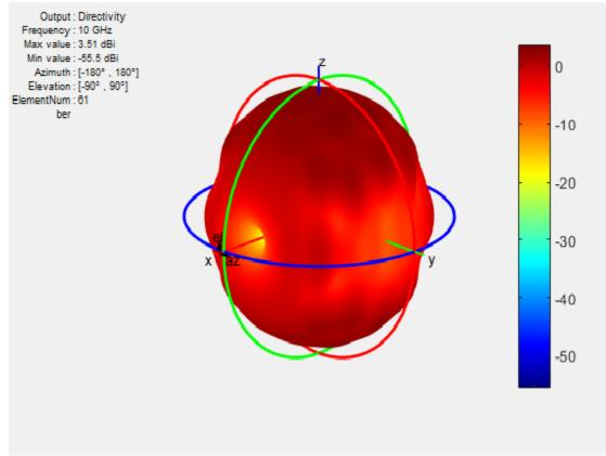
The figure shows the embedded element pattern of a center element in a 11x11 array. You can also calculate the embedded element pattern as a magnitude of electric field.
