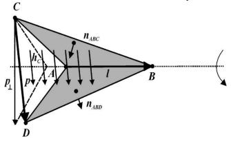
The figure shows an edge-based basis function. The vector variation is perpendicular to
