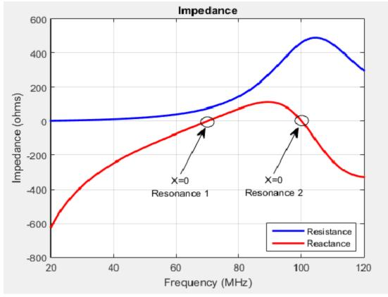
The plot shows two resonance points of a dipole antenna.
