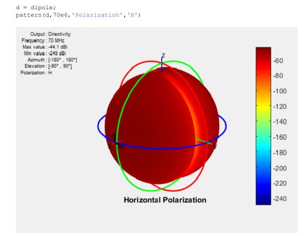
USA television networks use horizontally polarized antennas for broadcasting.
