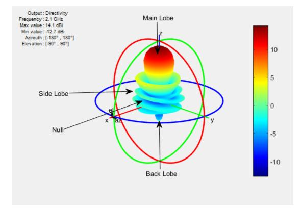
Use the pattern function to plot radiation pattern of any antenna in the Antenna Toolbox. By default, the function plots the directivity of the antenna. You can also plot the electric field and power pattern by using *Type* name-value pair argument of the pattern function.
