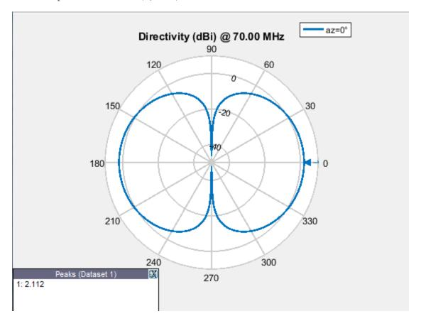
H-plane: Plane containing the magnetic field vector and the direction of maximum radiation. Use the patternAzimuth function to plot the azimuth plane pattern of a dipole antenna. The azimuthal variation in pattern shown captures the H-plane behavior of the dipole antenna.
