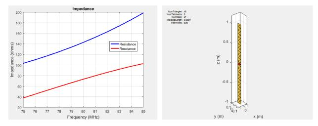
In above example, the dipole is meshed at the highest frequency, 85 MHz automatically before calculating the impedance at all the frequencies from 75 to 85 MHz. Meshing at the highest frequency, 85 MHz, ensures maximum number of triangles and a smoother plot of the dipole impedance. Use the mesh command to view the meshed dipole. The number of triangles is 48, which is more than single frequency meshing.
