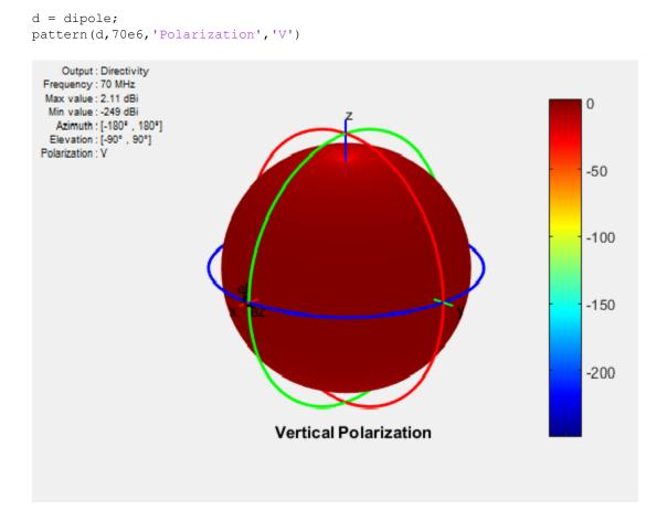
An AM radio broadcast antenna or an automobile whip antenna are some examples of vertically polarized antennas.
