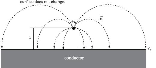
If you place a conducting object along this equipotential surface, then the field above the surface does not change.
