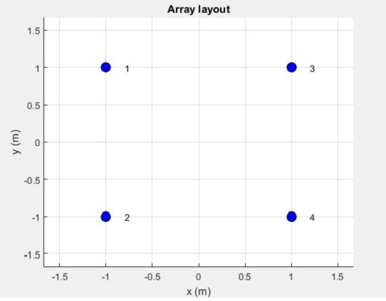
an element array arranged in a 2x2 grid. Visualize the grid and the element numbers using the layout.
