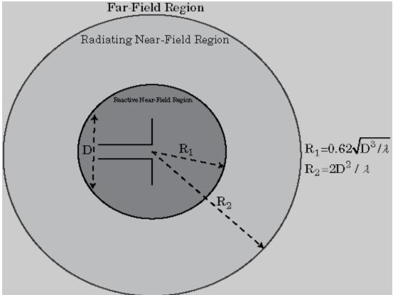
The region around an antenna is defined in many ways. The most used description is a 2or 3-region model. The 2-region model uses the terms *near field* and the *far field* to identify specific dominant field mechanisms. The diagram is a representation of antenna fields and boundaries. The 3-field region splits the near field into a transition zone, where a weakly radiative mechanism is at work.
