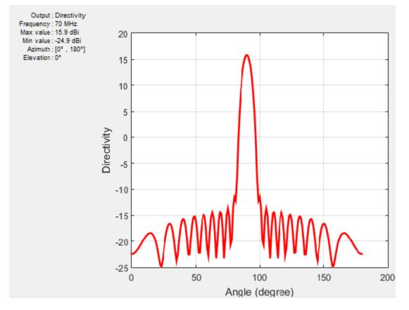
To scan the beam at a specific angle, use phase shift on the linear array:
