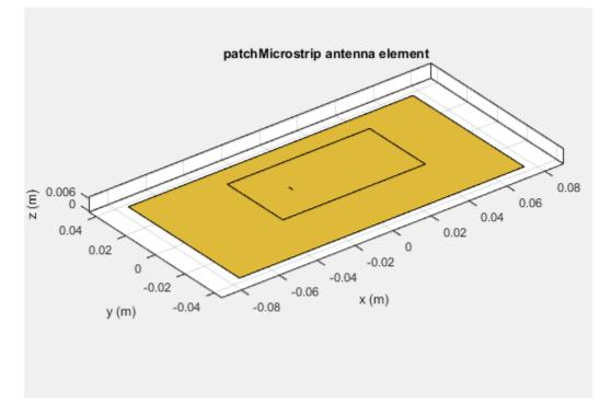
To make the antenna lie on the Y-Z plane, rotate it by 90 degrees about the Y-axis. The rotation follows the standard right-hand rule.
