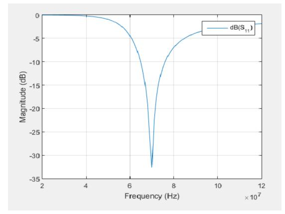
The reflection coefficient also gives the operating bandwidth of the antenna. Antenna bandwidth is usually the frequency band over which the magnitude of the reflection coefficient is below -10 dB.
